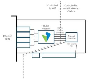
Versa Secure SD-NIC solution is a distributed solution. One or more SD-NIC can be placed in each compute appliance to provide a distributed and highly scalable L2, L3, L4-7 set of functions delivered from within each compute platform. SD-NIC based on VOS is then the Data Plane for all L2-L3, L4-L7 functions.
