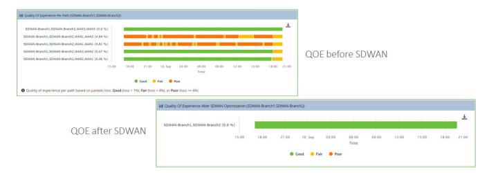
The quality of experience with SDWAN resulting from traffic steering, Forward Error Correction (FEC), replication
