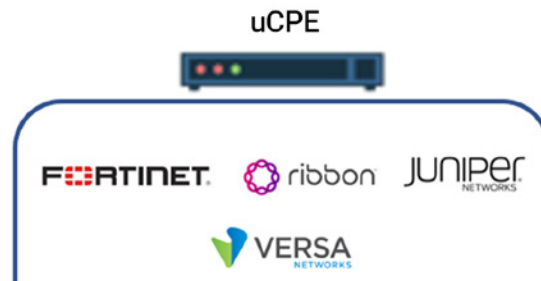
Figure 8 – Different network functions (firewalls, WAN optimization, authentication, et al.) can be implemented in uCPE, leveraging the VNFs of other vendors and minimizing equipment power and space utilization.
