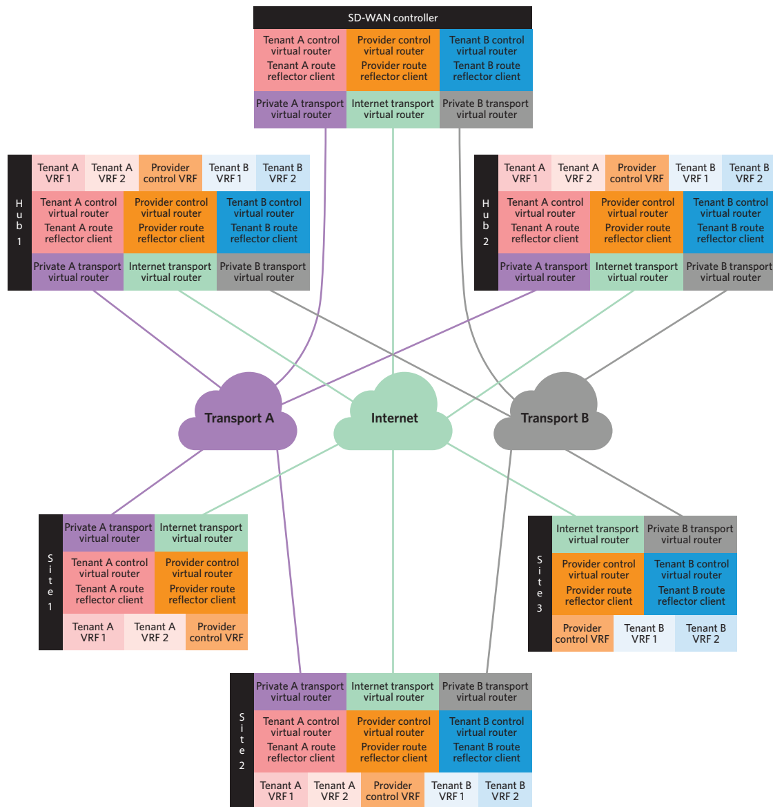
Figure 2 – Even if transport is shared, a proper multitenant architecture allows only the data that is pertinent to the tenant to be displayed or captured.
