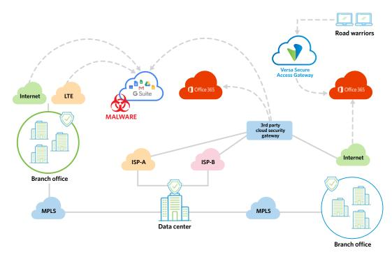
Fig. 2 - In a SaaS-ready architecture, a secure SD-WAN provides security at each location and network access point.
