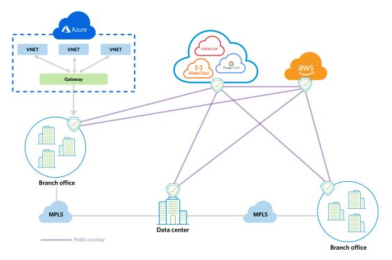
Fig. 3 – A secure SD-WAN seamlessly establishes dynamic overlay IPSec connectivity across disparate clouds for both the data and control planes.
