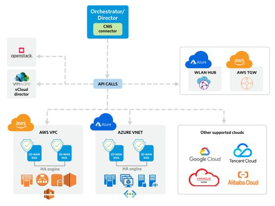
Fig. 4 - A secure SD-WAN supports integration with third-party cloud environments.
