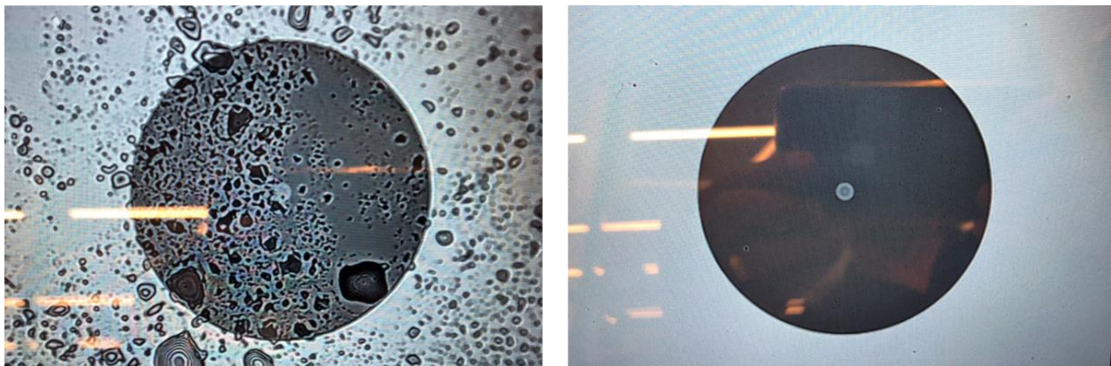
Figure 2 Dirty vs. clean Fiber Ferrule Tip
