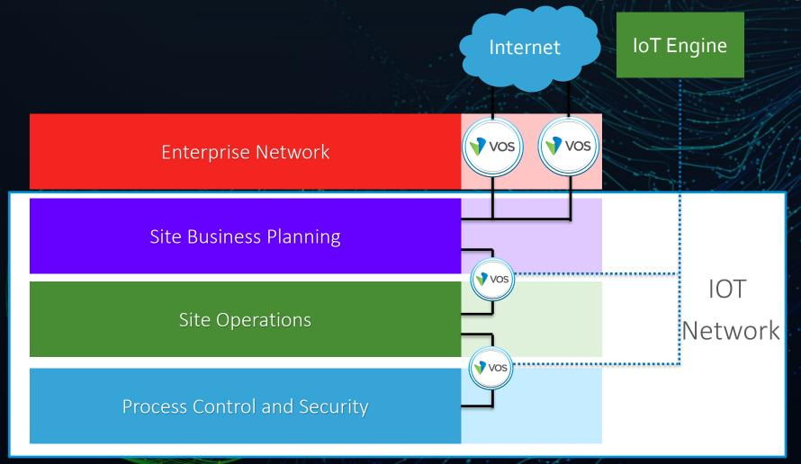
NGFW deployed deep inside the IOT/OT network to detect devices and to secure the network
