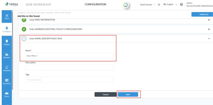
The screenshot shows the 'Add Site-to-Site Tunnel' configuration screen. The 'Enter NAME, DESCRIPTION & TAGS' section is highlighted with a red box. Inside this box, the 'Name' field contains 'Azure-IPsec-1'. Below the name field is a 'Description' field and a 'Tags' field, both of which are empty. At the bottom of the form are 'Cancel' and 'Save' buttons, with the 'Save' button also highlighted with a red box.
