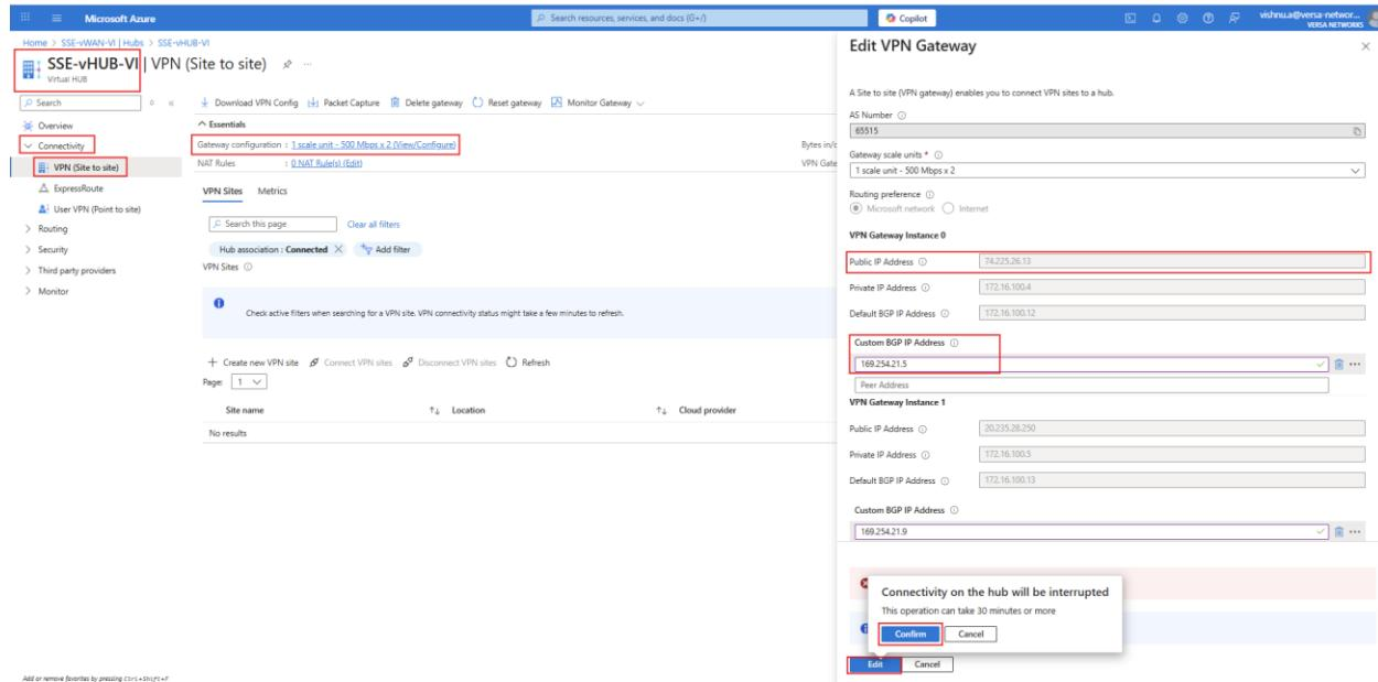
The screenshot shows the Microsoft Azure portal interface for managing a Virtual Hub. The left sidebar shows 'Virtual HUB' selected. Under 'Connectivity', 'VPN (Site to site)' is selected. The main pane shows 'Edit VPN Gateway' configuration. Key fields include:
