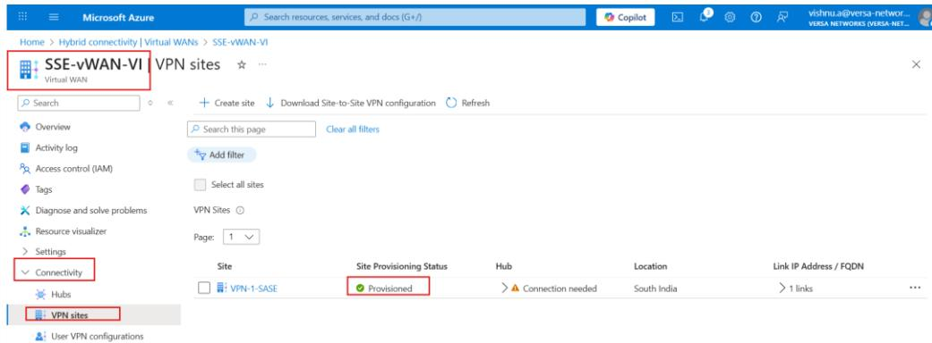
The screenshot shows the Microsoft Azure SSE-vWAN-VI VPN sites page. The 'VPN sites' tab is selected. A table lists a single VPN site: 'VPN-1-SASE' with a status of 'Provisioned'. The table columns are Site, Site Provisioning Status, Hub, Location, and Link IP Address / FQDN. The 'VPN sites' section in the left sidebar is also highlighted.
