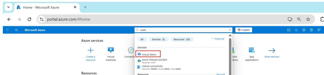
The screenshot shows the Microsoft Azure portal homepage. A search bar at the top right contains the text 'vwan'. Below the search bar, the 'Services' section is visible, with 'Virtual WANs' highlighted by a red box. Other services listed include 'Azure VMware Solution', 'Hybrid connectivity', and 'Enterprise connections'. The 'Virtual machines' and 'Connectivity' sections are also visible on the left.
