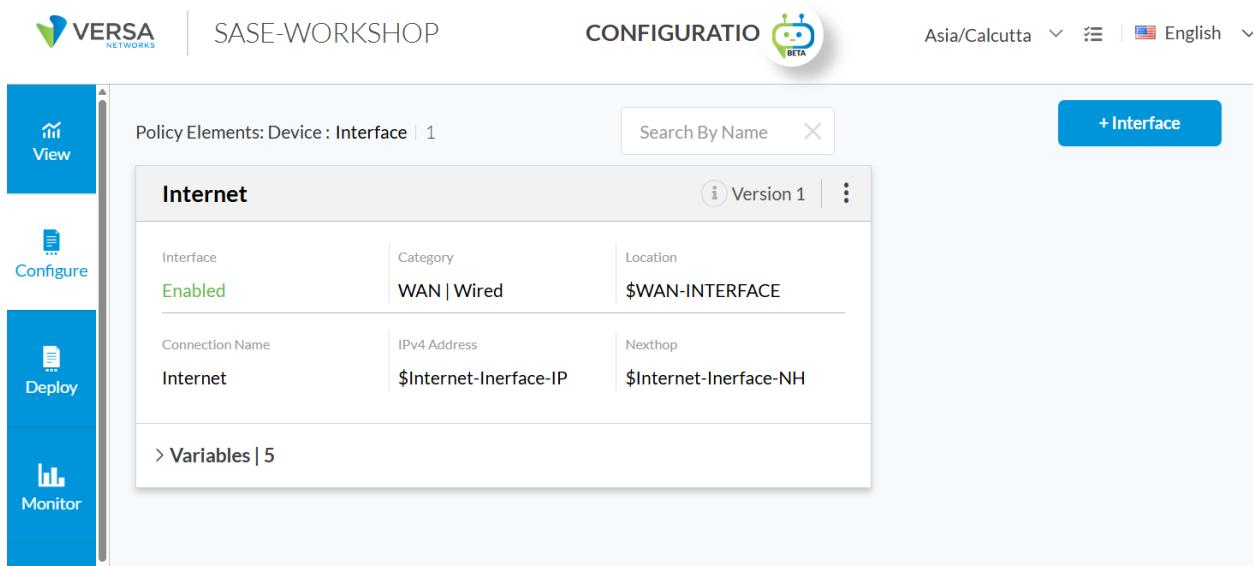
The screenshot shows the 'Policy Elements: Device : Interface' table with a single entry for 'Internet'. The 'Interface' column shows 'Enabled', 'Category' shows 'WAN | Wired', and 'Location' shows '\$WAN-INTERFACE'. The 'Variables' section shows 5 entries. A blue box highlights the 'Internet' entry in the table.
