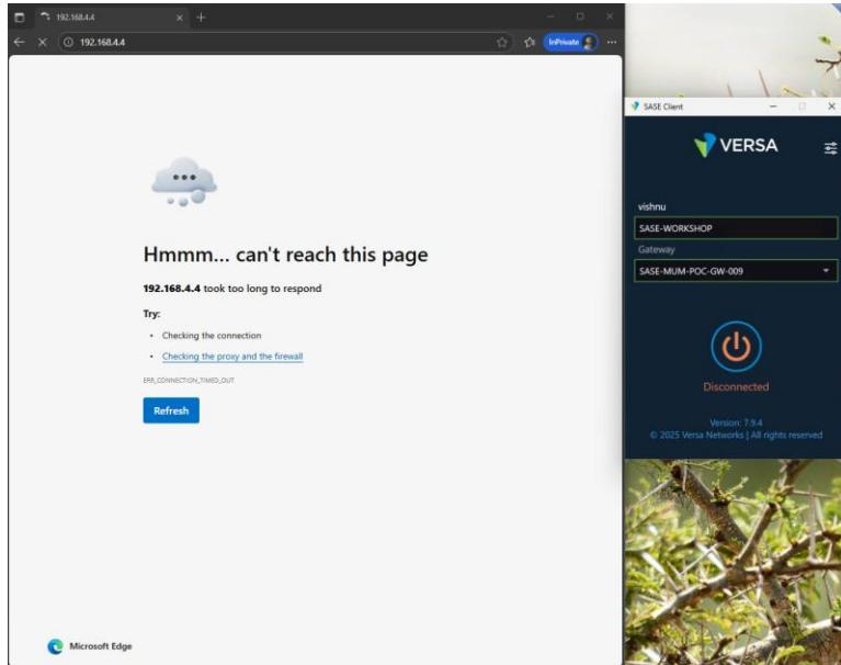
When the SASE Client is connected to the Gateway, we were able to reach the Azure VM instance over Private IP.
