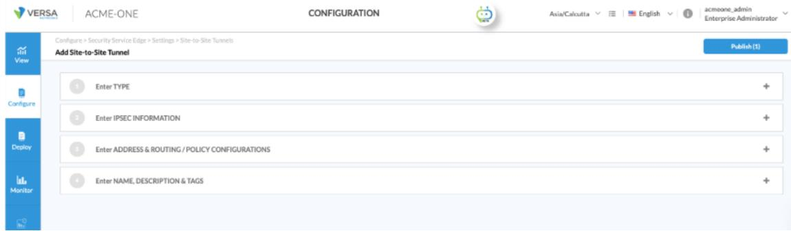
The default tunnel selection is IPsec. The remaining details, including tunnel type, remote address, and other parameters, should be configured as outlined below.
